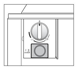
The controls consist of the temperature selector knob and the On/Off button. These are only visible when the drawer is open.
